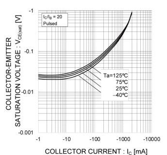
Fig.6 Collector-Emitter Saturation
