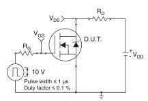
Fig. 13 - Switching Time Test Circuit
