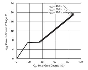
Fig. 7 - Typical Gate Charge vs. Gate-to-Source Voltage
