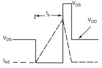
Fig. 16 - Unclamped Inductive Waveforms
