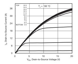
Fig. 2 - Typical Output Characteristics
