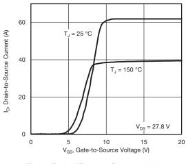
Fig. 3 - Typical Transfer Characteristics
