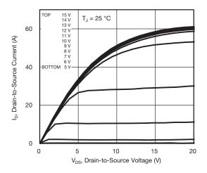
Fig. 1 - Typical Output Characteristics
