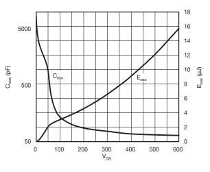
Fig. 6 -  $C_{\text{OSS}}$  and  $E_{\text{OSS}}$  vs.  $V_{\text{DS}}$
