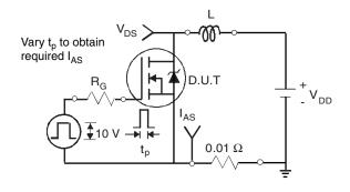
Fig. 15 - Unclamped Inductive Test Circuit
