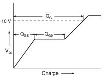
Fig. 17 - Basic Gate Charge Waveform
