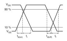
Fig. 14 - Switching Time Waveforms
