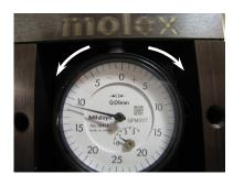
Shut height is less than 135.8mm
