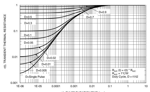
t1, PULSE DURATION TIME (sec) Figure 13. Transient Thermal Resistance
