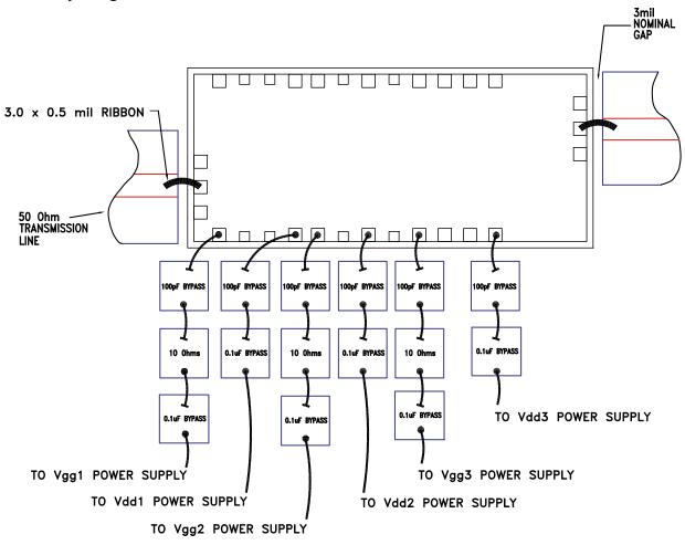
Note 1: Bypass caps should be 100 pF (approximately) ceramic (single-layer) placed no farther than 30 mils from the amplifier.
