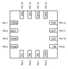
3mm x 3mm MLF<sup>®</sup> (ML) Fixed DC/DC Converter Output Voltage
