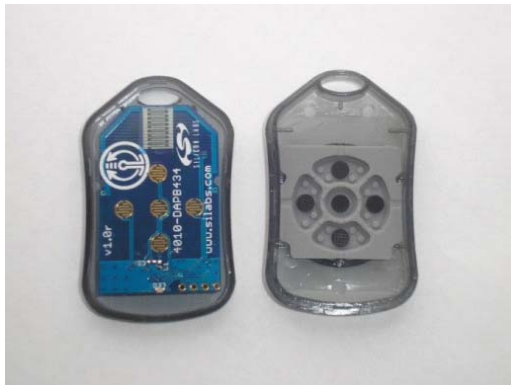
Figure 1. Si4010 Universal Key Fob and Plastic Case (P/N 4010-DAPB 868 and MSC-PLPB_1)
