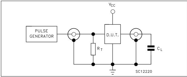
$C_L$  = 50pF or equivalent (includes jig and probe capacitance)  $R_T$  =  $Z_{OUT}$  of pulse generator (typically 50 $\Omega$ )
