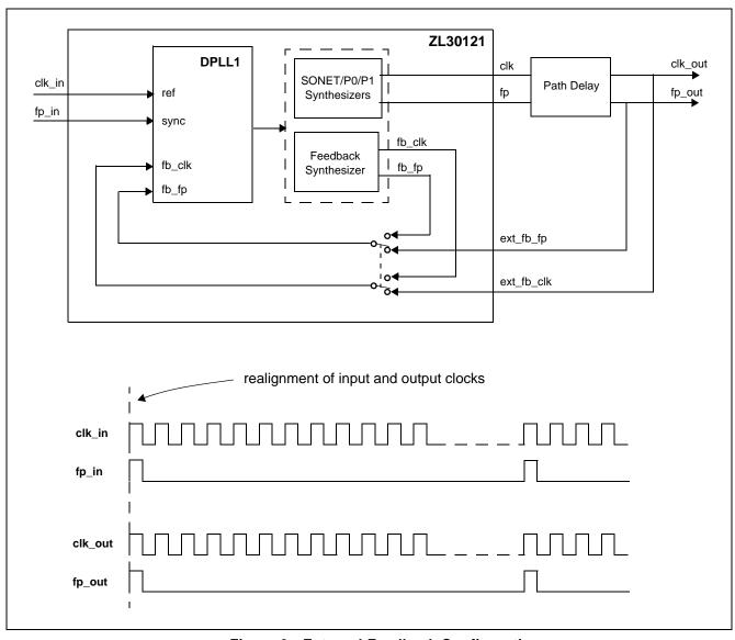
Figure 9 - External Feedback Configuration
