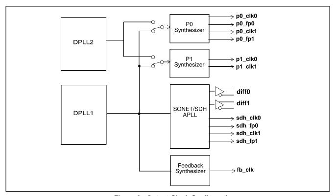
Figure 6 - Output Clock Configuration
