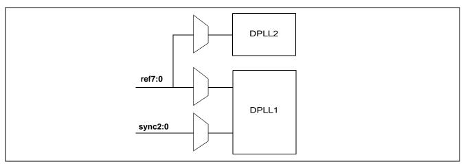
Figure 3 - Reference and Sync Inputs
