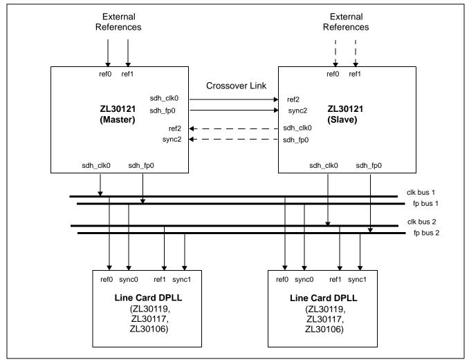
Figure 8 - Typical Master/Slave Configuration
