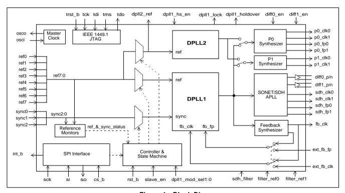
Figure 1 - Block Diagram
