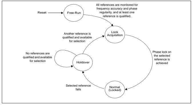
Figure 2 - Automatic Mode State Machine
