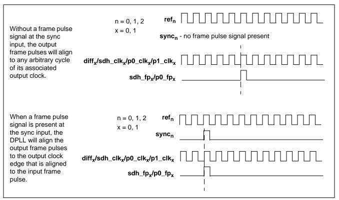
Figure 4 - Output Frame Pulse Alignment
