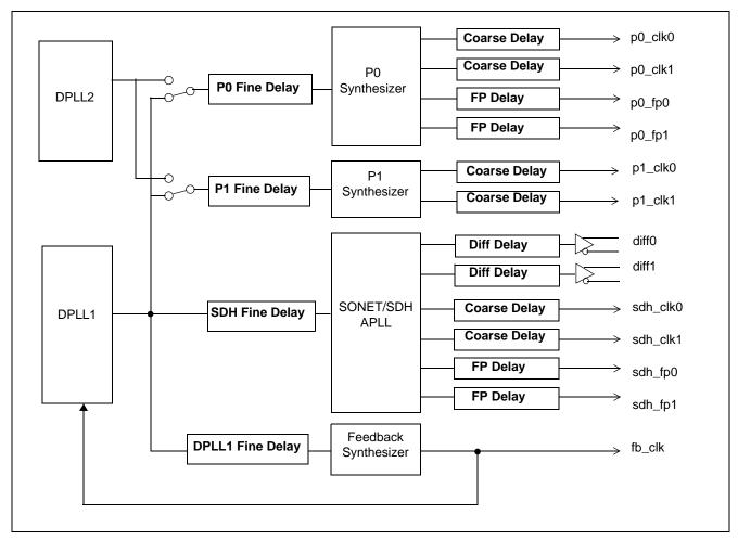
Figure 7 - Phase Delay Adjustments
