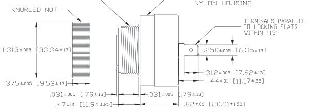
MOUNTING: REMOVE BLACK PLASTIC NUT AND INSERT THREADED FRONT THROUGH 1.25"
