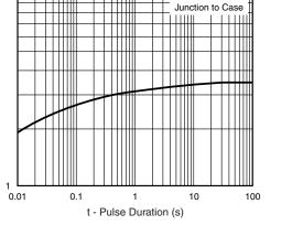
Fig. 5 - Typical Transient Thermal Impedance Per Diode
