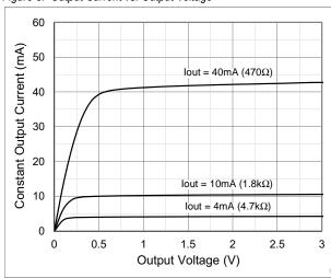
Figure 4. ICOC vs. Supply Voltage; REXT =  $470\Omega$
