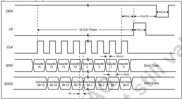
Figure 12. Data Input Example Timing Diagram
