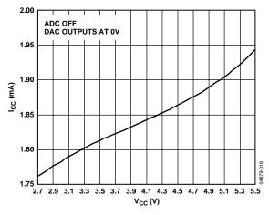
Figure 18. Supply Current vs. Supply Voltage @ 25℃
