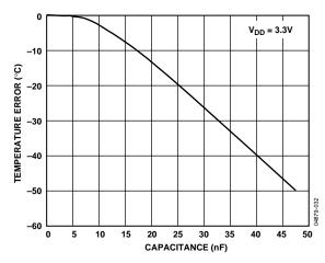
Figure 32. External Temperature Error vs. Capacitance between D+ and D-
