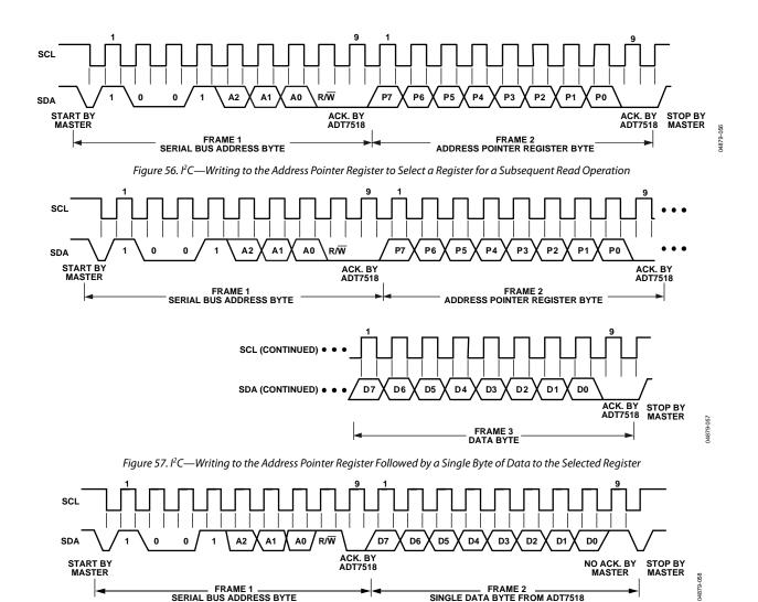
Figure 58. I<sup>2</sup>C—Reading a Single Byte of Data from a Selected Register
