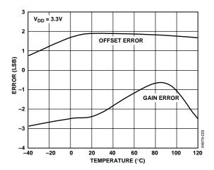
Figure 29. ADC Offset Error and Gain Error vs. Temperature
