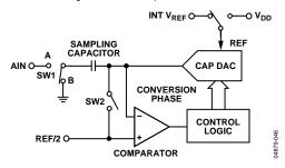
Figure 46. ADC Conversion Phase
