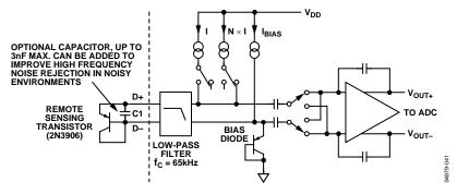
Figure 41. Signal Conditioning for External Diode Temperature Sensor
