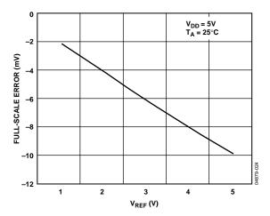
Figure 24. DAC Full-Scale Error vs. VREF
