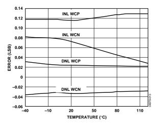
Figure 13. ADT7518 DAC INL Error and DNL Error vs. Temperature
