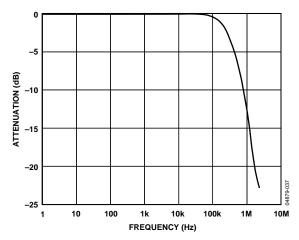
Figure 37. DAC Multiplying Bandwidth (Small Signal Frequency Response)
