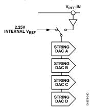
Figure 40. DAC Reference Buffer Circuit
