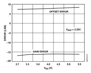
Figure 15. DAC Offset Error and Gain Error vs.  $V_{\text{DD}}$
