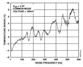
Figure 33. External Temperature Error vs. Common-Mode Noise Frequency
