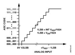
Figure 47. Single-Ended Transfer Function
