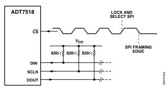
Figure 55. Typical SPI Interface Connection
