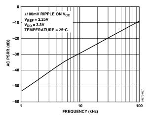
Figure 27. PSRR vs. Supply Ripple Frequency
