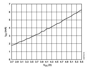
Figure 19. Power-Down Current vs. Supply Voltage @ 25°C
