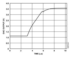
Figure 20. DAC Half-Scale Settling (1/4 to 3/4 Scale Code Change)
