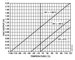
Figure 43. DAC Output vs. Temperature  $V_{REF}$ -IN = 2.25 V
