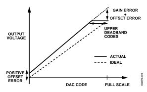
Figure 9. DAC Transfer Function with Positive Offset ( $V_{REF} = V_{DD}$ )
