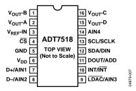
Figure 7. Pin Configuration QSOP
