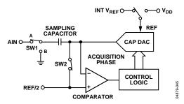
Figure 45. ADC Acquisition Phase
