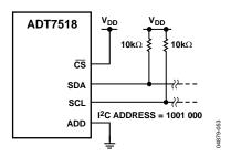
Figure 54. Typical I<sup>2</sup>C Interface Connection
