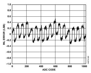
Figure 26. ADC INL with Ref =  $V_{DD}$  (3.3 V)
