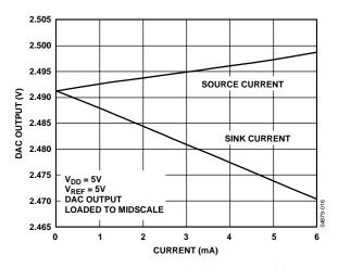
Figure 16. DAC V<sub>OUT</sub> Source and Sink Current Capability
