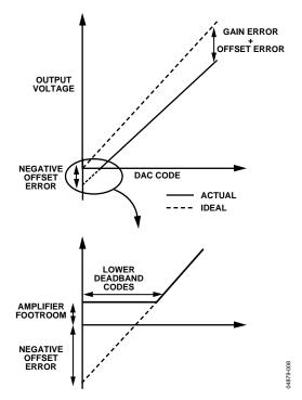
Figure 8. DAC Transfer Function with Negative Offset
