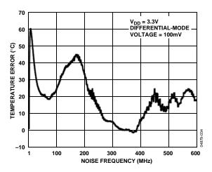
Figure 34. External Temperature Error vs. Differential-Mode Noise Frequency
