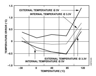
Figure 28. Internal Temperature Error @ 3.3 V and 5 V
