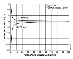
Figure 31. External Temperature Error vs. PCB Leakage Resistance
