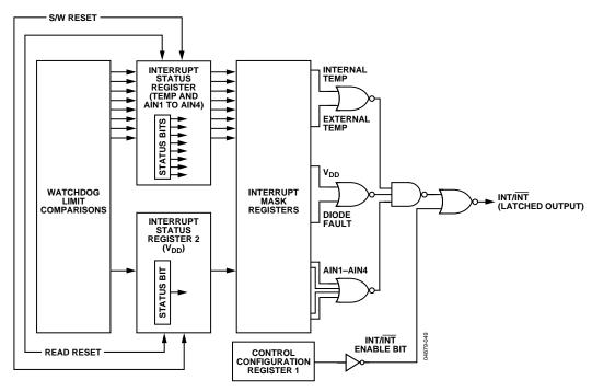
Figure 49. Interrupt Structure
