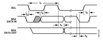
Figure 2. I<sup>2</sup>C Bus Timing Diagram
