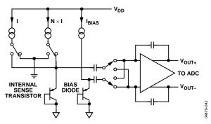
Figure 42. Top Level Structure of Internal Temperature Sensor
