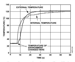
Figure 36. Temperature Sensor Response to Thermal Shock
