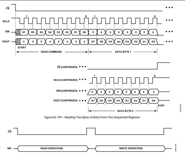
Figure 63. SPI—Correct Use of CS During SPI Communication
