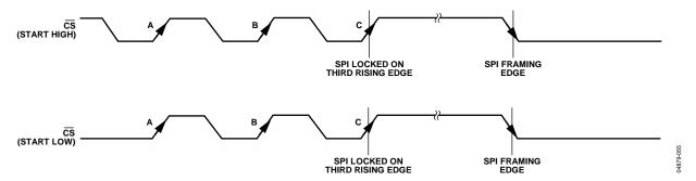
Figure 53. Serial Interface—Selecting and Locking SPI Protocol
