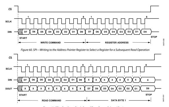
Figure 61. SPI—Reading a Single Byte of Data From a Selected Register
