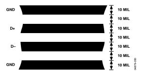
Figure 50. Arrangement of Signal Tracks
