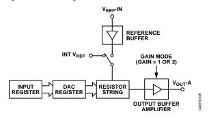
Figure 38. Single DAC Channel Architecture
