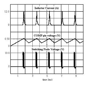
Figure 6. Hiccup Overcurrent Protection
