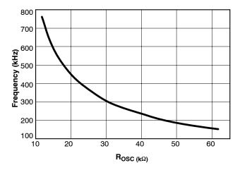
Figure 8. Switching Frequency
