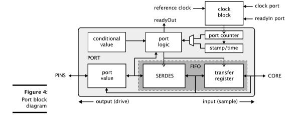
ports are available. All pins of a port provide either output or input. Signals in different directions cannot be mapped onto the same port.
