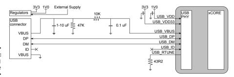
Figure 12: Self powered USB-device
