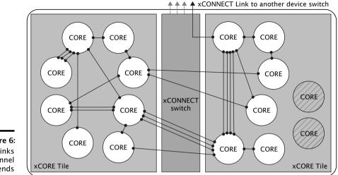
Figure 6: Switch, links and channel ends
