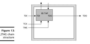
The JTAG chain structure is illustrated in Figure 13. It comprises a single 1149.1 compliant TAP that can be used for boundary scan of the I/O pins. It has a 4-bit IR and 32-bit DR. It also provides access to a chip TAP that in turn can access the xCORE Tile for loading code and debugging.
