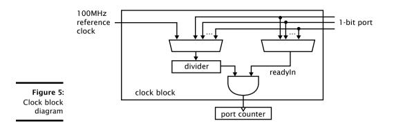
A clock block can use a 1-bit port as its clock source allowing external application clocks to be used to drive the input and output interfaces. xCORE-200 clock blocks optionally divide the clock input from a 1-bit port.
