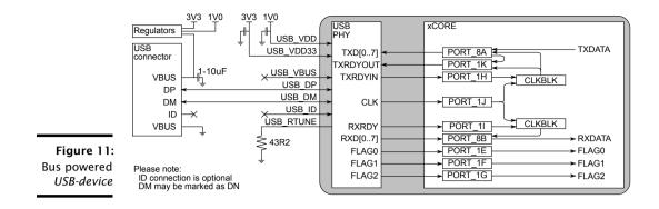
An external resistor of 43.2 ohm (1% tolerance) should connect USB\_RTUNE to ground, as close as possible to the device.
