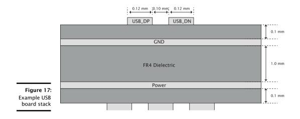
We recommend that the high-speed clock and high-speed USB differential pairs are routed first before any other routing. When routing high speed USB signals, the following guidelines should be followed:
