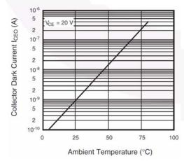
Figure 5. Collector Dark Current vs. Ambient Temperature
