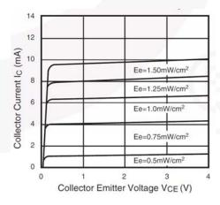
Figure 6. Collector Current vs. Collector Emitter Voltage
