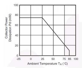
Figure 1. Collector Power Dissipation vs. Ambient Temperature
