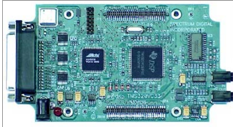
eZdsp™ for TMS320VC33 with eZdsp VC33 Code Composer
