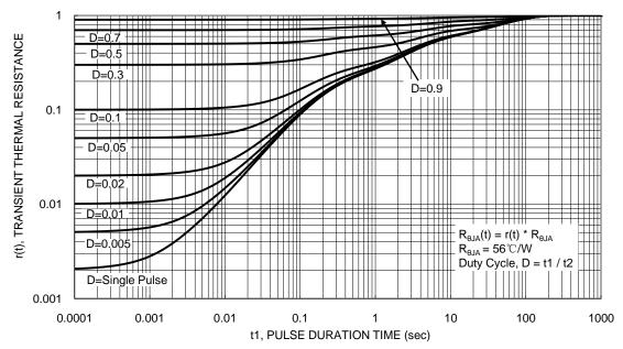
Figure 13. Transient Thermal Resistance
