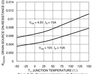
Figure 7. On-Resistance Variation with Temperature
