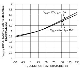
Figure 6. On-Resistance Variation with Temperature
