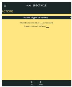
Trigger an action when a button is released, regardless of how long it has been held down prior to being released.
