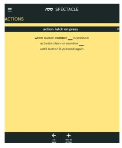
Here are the settings we need to use for this project. We want button 8 (the button on the Button Board) to activate channel 0 when pressed. Later on, we'll tell our light board to watch channel 0 and do something when it's active.
