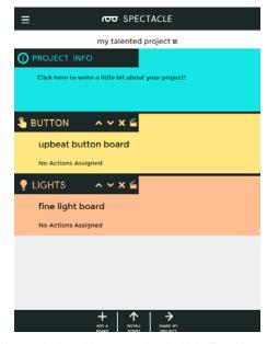
Each board has a clapboard icon associated with it. To add or edit actions, click this icon. We're going to start by adding an action to the button board.
