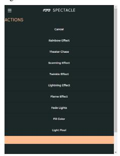
The Light board supports 9 different actions. Most of them want a continuous-type signal input, although a couple of them can be used with momentary input signals. We'll cover the difference under each action. Each action will have a field for the number of pixels the lightstrip that action is being applied to has, and we won't mention it again.
