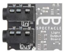
The Light Board supports up to three strands of addressable LEDs. Each strand can have up to 60 individual pixels. **Not all types of addressable LEDs are compatible with the Spectacle Light Board**. If you have questions about whether or not a particular type of LED strip is compatible with the Light Board, contact SparkFun technical support.
