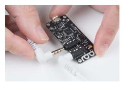
Take the other end of this cable and plug it into the audio jack of the phone, tablet, or computer that you'll be using to program the system.
