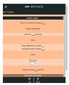
Turns on one light and blanks the rest of the lights to off.
