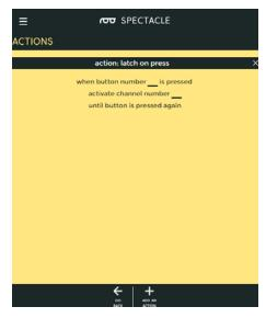
This action is like a latching power switch. One press turns the signal on, another later press turns the signal off.
