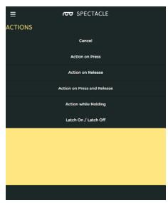
For the Button board, there are five options: three which produce a momentary pulse type output and two that produce a continuous switch type output.
