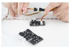
Finally, plug the Micro B end of the power adapter into the Director Board, and the other end into the wall. You should see one solid light and one blinking light on the Light board and the Button board. On the Director Board, you'll see one solid light and one light which blinks eight times, then pauses, then repeats. This shows that power is present and the boards are up and running.
