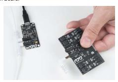
Grab another of the TRRS cables and plug it into the "Out" jack on the Button Board.
