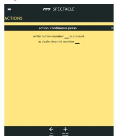
Trigger an event as soon as a button is pressed, then continue to trigger that event as long as the button is held down.
