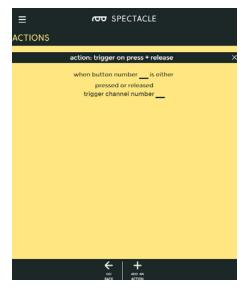
Trigger an action when a button is pressed, then trigger the same action again when the button is released.
