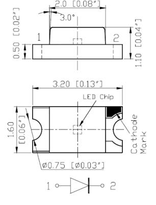
Units: mm / tolerance = +/-0.1mm
