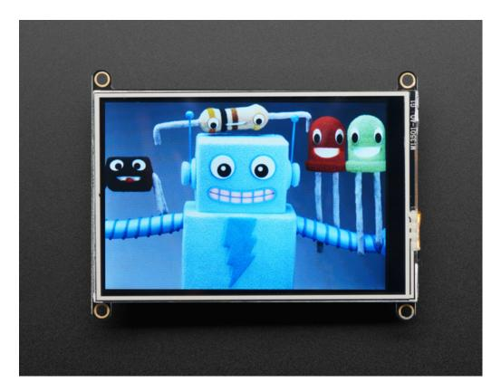
To make new bitmaps, make sure they are less than 480 by 320 pixels and save them in **24-bit BMP format!** They must be in 24-bit format, even if they are not 24-bit color as that is the easiest format for the Arduino. You can rotate images using the **setRotation()** procedure
