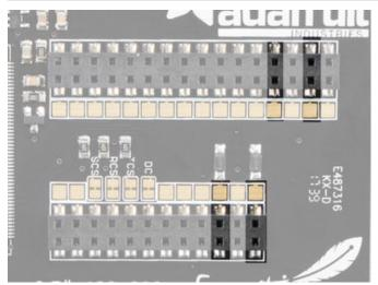
The 3.5" TFT FeatherWing has a really beefy backlight, and we don't want to overwhem the 3.3V regulator on the Feather so we use two Schottkey diodes to take the higher of **VBAT** and **VUSB** to feed into the backlight boost converter.
