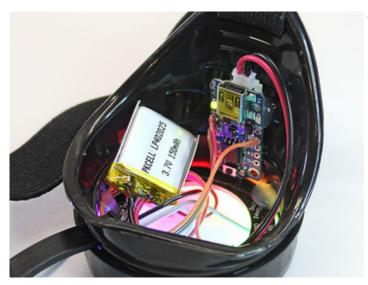
The battery is small enough to tuck away inside the eye cup. Add a bit of masking tape to hold it in place if needed.
