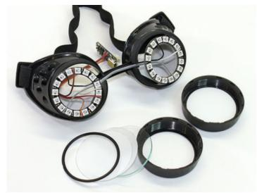
Insert the electronics into the goggles from the front, with the ring-to-ring ribbon cable across the bridge of the nose.
