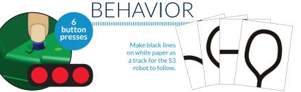
STEP 1: Print out a set of black lines from the "Tracks.pdf" (Download file from www.parallax.com/go/S3). Do not use photograph printing ink, which reflects infrared light!
