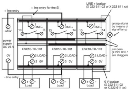
Application examples: line entry DC 24 V with protection of signal circuit and direct connection of loads
