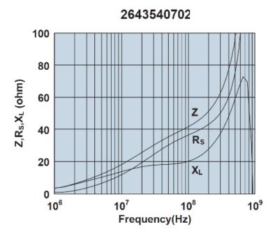
Impedance, reactance, and resistance vs. frequency.
