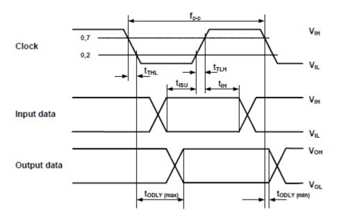
Figure 3.1: SDIO/SPI timing diagram (default mode)
