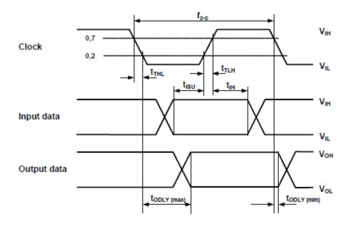
Figure 3.1: SDIO/SPI timing diagram (default mode)
