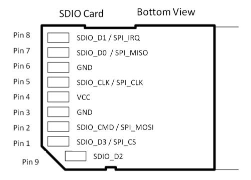
Figure 4.1: SPB104 pinout. bottom view
