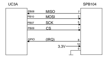
For some host systems the only communication method is the SPI mode (EVK1105). In these systems the host processor must poll the SPB104 regularly to communicate. If better latency is required, an interrupt line is available on the side of the SPB104 board. This line could be connected to an appropriate interrupt line on the host system.
