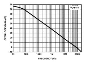
FIGURE 1. OPEN-LOOP GAIN vs FREQUENCY
