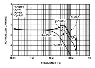
FIGURE 9. GAIN vs FREQUENCY FOR VARIOUS  $R_{LOAD}$  (A<sub>V</sub> = +1)
