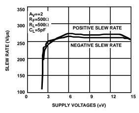
FIGURE 8. SLEW RATE vs SUPPLY
