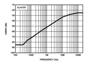
FIGURE 17. COMMON-MODE REJECTION RATIO (CMRR)
