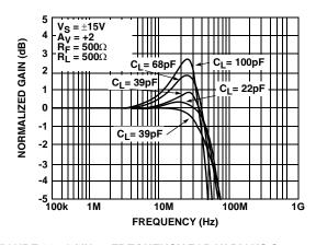
FIGURE 12. GAIN vs FREQUENCY FOR VARIOUS  $C_{LOAD}$ (A<sub>V</sub> = +2)
