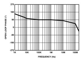
FIGURE 2. OPEN-LOOP PHASE vs FREQUENCY
