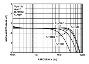
FIGURE 10. GAIN vs FREQUENCY FOR VARIOUS  $R_{LOAD}$  ( $A_V = +2$ )
