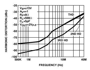
FIGURE 19. HARMONIC DISTORTION vs FREQUENCY  $(A_V = +1)$
