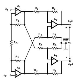
FIGURE 30. DIFFERENTIAL OUTPUT AMPLIFIER
