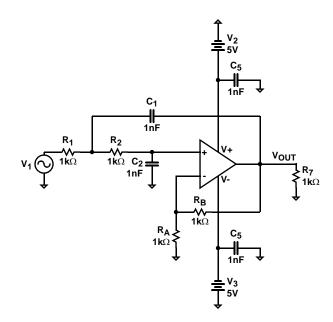
$$\begin{aligned} & \text{Holp} = K \\ & \text{wo} = \frac{1}{\sqrt{\text{R1C1R2C2}}} \\ & \text{Q} = \frac{1}{(1 - K)\sqrt{\frac{\text{R1C1}}{\text{R2C2}}} + \sqrt{\frac{\text{R1C2}}{\text{R2C1}}} + \sqrt{\frac{\text{R2C2}}{\text{R1C1}}} \end{aligned}$$
