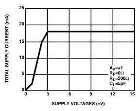
FIGURE 25. SUPPLY CURRENT vs SUPPLY VOLTAGE
