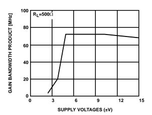
FIGURE 7. GAIN BANDWIDTH PRODUCT vs SUPPLY
