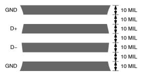
Figure 19. Arrangement of Signal Tracks
