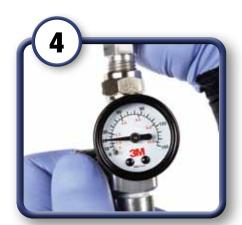
Set air pressure at 20 psi at full trigger (air and fluid flowing).
