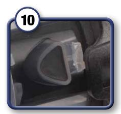
Inspect atomizing head for damage or wear which could result in fluid leaks or poor performance.
