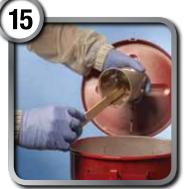
Remove unused material from the liner and place into proper disposal container.
