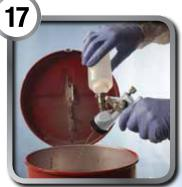
A squeeze bottle (PN 37720) containing solvent or water enables fast gun cleaning once the 3M<sup>™</sup> PPS<sup>™</sup> cup is removed. More efficient painters make facility more productive.
