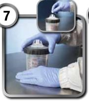
Position locking collar onto the 3M<sup>™</sup> PPS<sup>™</sup> cup/liner and turn until tight. Insert sealing plug prior to shaking.
