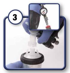
Attach 3M<sup>™</sup> PPS<sup>™</sup> cup filled with coating and attach compressed air hose.
