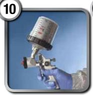
The spray gun is now ready to spray as normal. **NOTE:** For spraying upside-down, follow directions in the "Tips" section on purging air.
