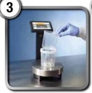
Remove liner from wall dispenser and place into 3M<sup>™</sup> PPS<sup>™</sup> mixing cup. Weigh the paint according to paint manufacturer's guidelines.
