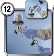
To return material back into gun cup before disconnecting spray gun, disconnect air line, invert gun (gravity feed only) and pull trigger fully for a few seconds.
