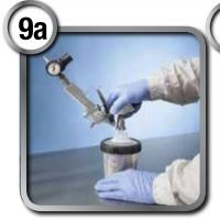
Spray gun with correct adapter is attached with a quick quarter turn.
