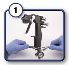
Hand tighten or use two wrenches to connect the air flow control value.
