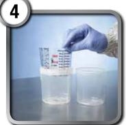
If not using a scale to measure, insert 3M<sup>™</sup> PPS<sup>™</sup> mix ratio film into cup before inserting liner in order to measure the paint according to paint manufacturer's quidelines.
