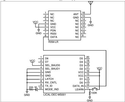
The Keyfob is set to 9,600bps, so SEL\_BAUD0 should be tied high and SEL\_BAUD1 tied low.
