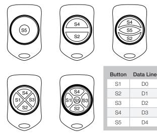
Figure 6: OTX-\*\*\*-HH-KF#-MS Button Assignments
